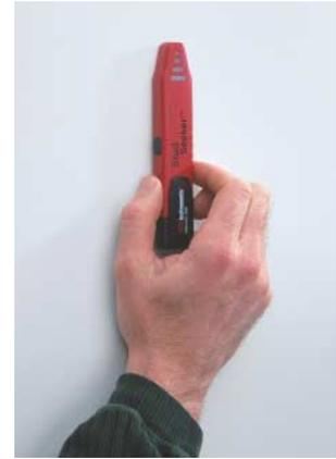
*Stud sensor: Indispensable tool for finding the right places to mount speakers, wall plates and controls.*
